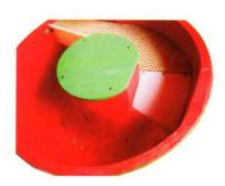
Bump Machine is designed for deburring, polishing, descaling, and antique finishing of any type of metal. It is preferred for heavy duty vibratory action on medium to large size parts. It has a curve wall bowl with 100% separation and manufactured by using cutting edge technologies.
